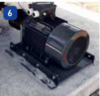
Electric drives Robust electric motors (equipped with a spur gear system depending on the application) transfer the output to a planetary bevel gear via a drive shaft. The drives are available in performance classes 22, 30 and 45 kW.
