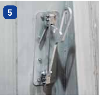
Mechanical shear bar The individually adjustable shear bars interrupt, when necessary, substrate rotation, thus supporting the optimal mixing of contents.
