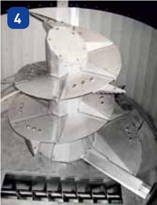
Vertical mixing screw With a speed of 8-12 r/min, the mixing screws ensure needs-based processing of substrates and subsequently transfer them to the conveyance technology. Different vertical mixing screws are available according to material and container volume, in either steel or stainless steel. The speed can be controlled with a frequency converter.
