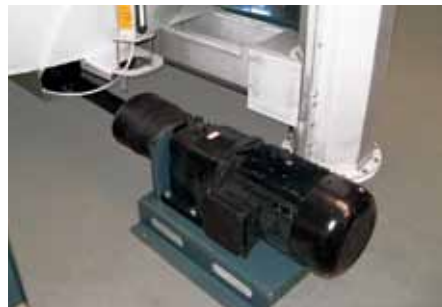
Driven via motor, drive shaft and planetary bevel gear to blade or mixing screw
