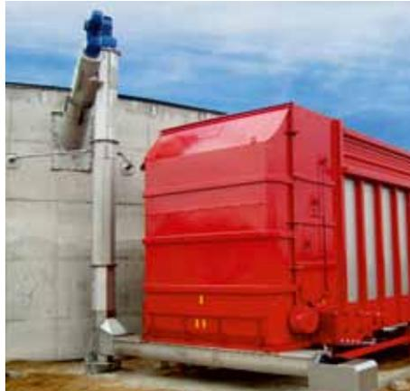
**Conveyor section model 360 with double base frame screw**
