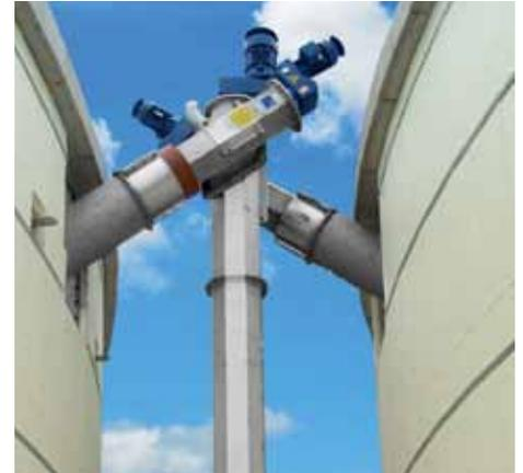
**Steep conveyor screw model 360 with 2 fermentation screws for double entry for 2 containers**
