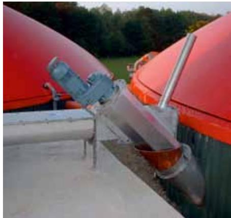
**Base frame screw and fermenter screw model 360 for floor grade input**
