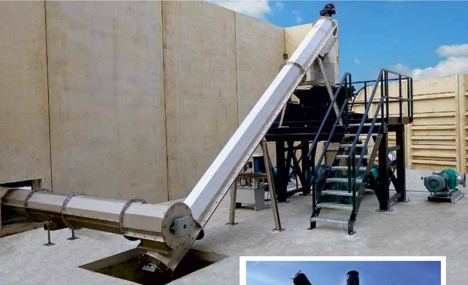
Screw section model 450 with horizontal and inclined screw conveyance to a crusher unit
