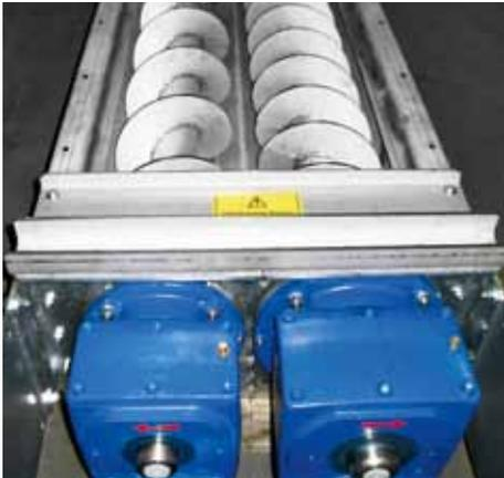
**Double base frame screw model 360 for taking in material from the push floor systems etc.**
