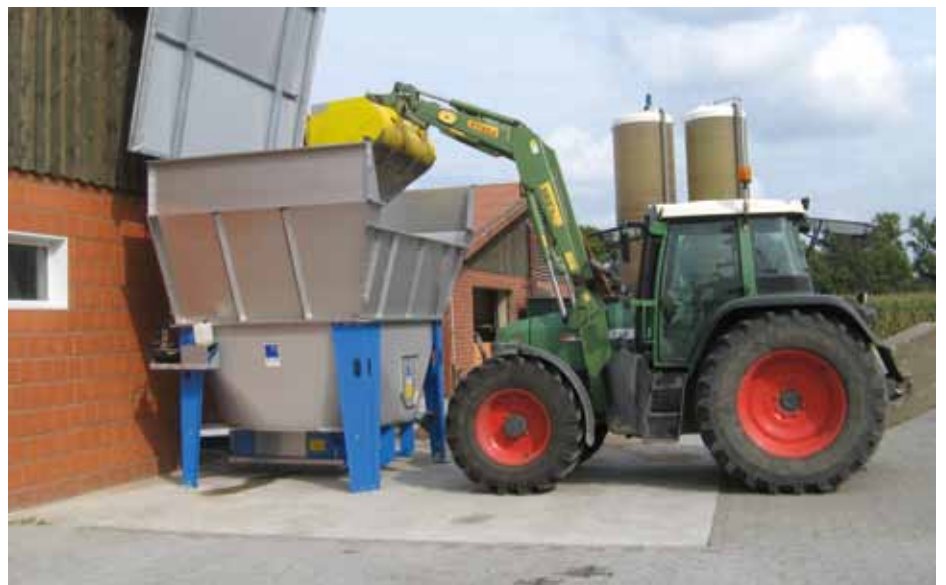
UNI-Dos model 200 with 20 m 3 storage volume, horizontal discharge screw model 160 and hydraulically operated cover
